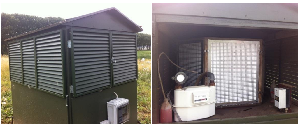
Figure 2.2 Aerosol sampler (left for external view and right for internal view) at Risø campus of Technical University of Denmark, Roskilde.
