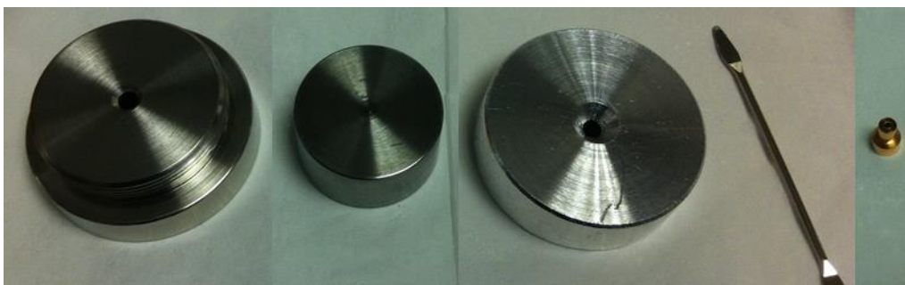
Figure 2.3 Picture of pressing tool for target preparation in the SUERC AMS lab, UK. The yellow component (the right most one) is the copper holder.
