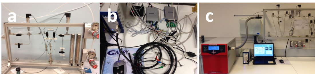
FIGURE A.3: The DEMS setup was constructed in two phases. To gain experience, we constructed a manual DEMS setup to determine appropriate volumes, flushing times etc. After this, we automated the setup in a Labview interface, basically making DEMS measurements a one-click experiment.
