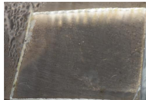
Flat antifog treated PMMA at 70% RH
