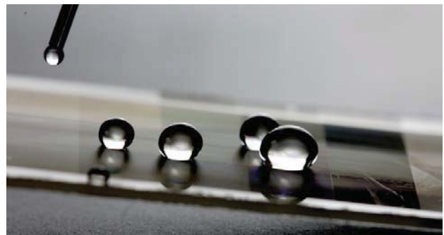
Figure 1: Drops on slightly tilted surface, excellent superhydrophobic properties.
