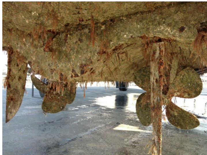
Figure 1.4. Example of bio-fouling 8 . Drag will be increased dramatically. Self-cleaning surfaces may prevent this.
