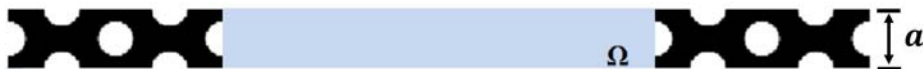
Figure 12: Slow light waveguide problem: a single design unit in a (vertically) periodic structure, design domain \Omega .
