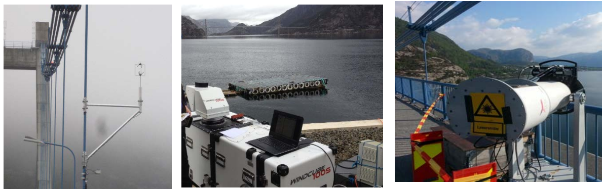
Figure 2. 3D WindMaster Pro fitted to a bridge hanger (left), WindCube 100S at the Lysefjord Center with the bridge in the background (middle) and one of the two short-range WindScanner lidars (R2D1) at the bridge walkway (right).
