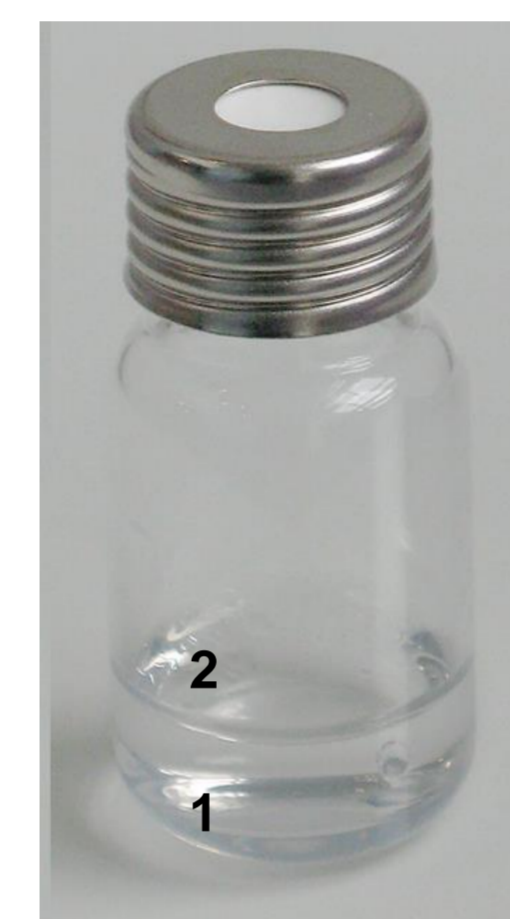
Figure 1. Passive dosing experiments. 1: Pyrethroid loaded silicone and 2: Equilibrated water with Daphnia magna .
