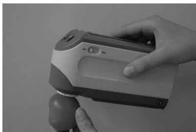
Figure 2.4: View of a spectrophotometer measuring the light diffusely reflected from a fruit (Bernd Herold, 2008)
