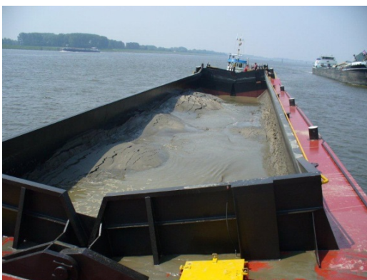
Figure 2.14 Dredged material ready to dumped from a split hopper, Right: The sediment plume due to dispersion and mixing of fine material after dumping
