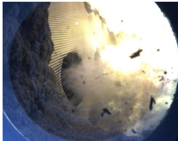
Figure 4: Side port view with flame detachment and flame stabilization approximately 1 meter into the furnace.
