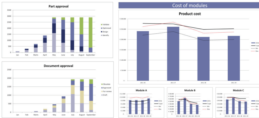
Figure 6. Example of reports showing design progress and cost development generated from the PLM system on a weekly basis
