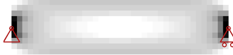
Fig. 1: Result obtained using the optimization formulation in Eq. (1) with a linear interpolation between the material properties of S1 (white) and titanium (black). The design mesh consists of 40 \times 10 elements, and the finite element mesh of 80 \times 20 elements.
