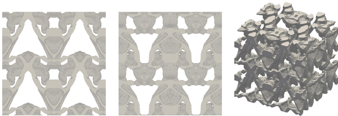
Figure 3.3: Another example of a microstructure with a negative Poisson's ratio (obtained with a volume constraint of 20%). The microstructure is illustrated by showing 2 \times 2 \times 2 unit cells together; from two perpendicular directions and one angled viewpoint.
