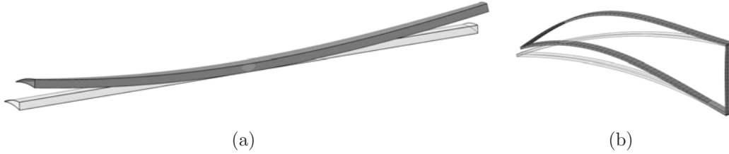
Figure 11: (a) Global deformation of the main beam model for a loading angle of \alpha = 135^\circ at \kappa = 0.01 \text{ m}^{-1} ; (b) in-plane deformation at mid-span for the same load case with a deformation scaling factor of 10.
