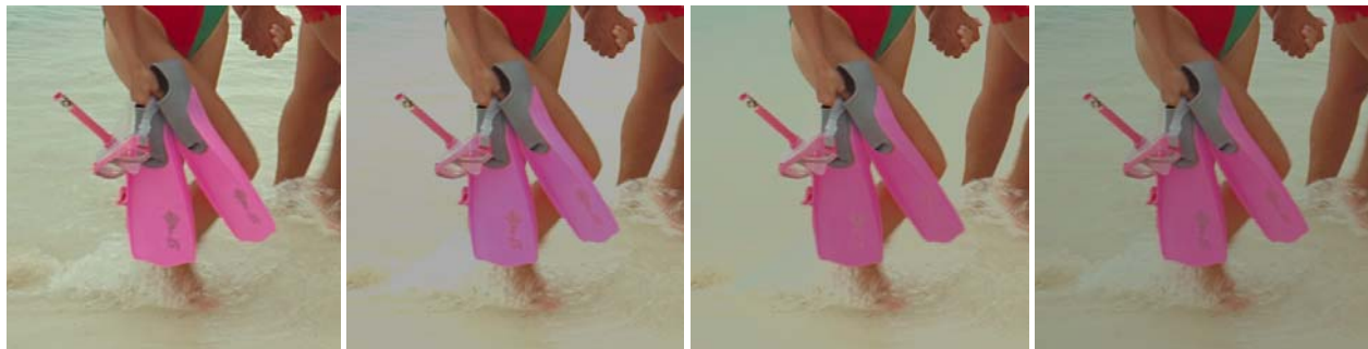
a) Original (full backlight) b) Hard clipping c) Hard + hue preservation d) Soft clipping
