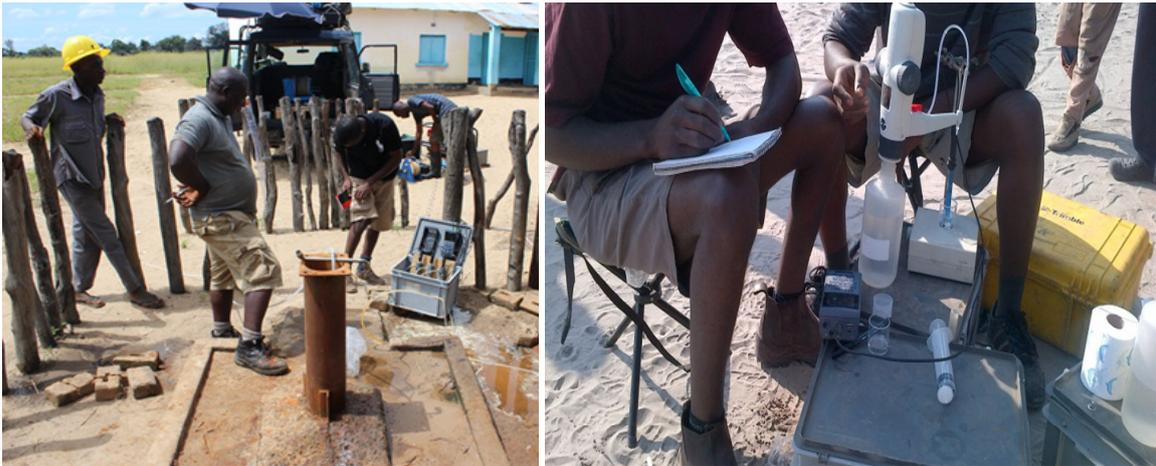
**Fig. 6:** Infield measurement involved opening of the production wells, measuring the groundwater level, physico-chemical measurements (pH, EC, DO and temperature) and alkalinity using the gran titration
