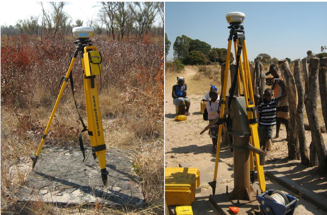
**Fig. 5:** Typical differential GPS setup with receivers at the base station and borehole site of interest.
