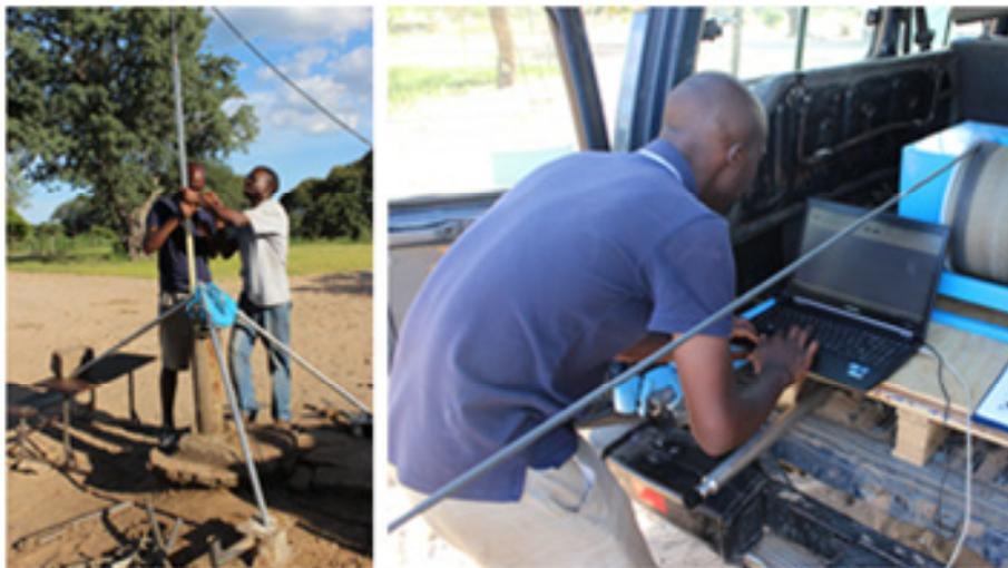
**Fig. 7:** Geophysical borehole logging during a field campaign.
