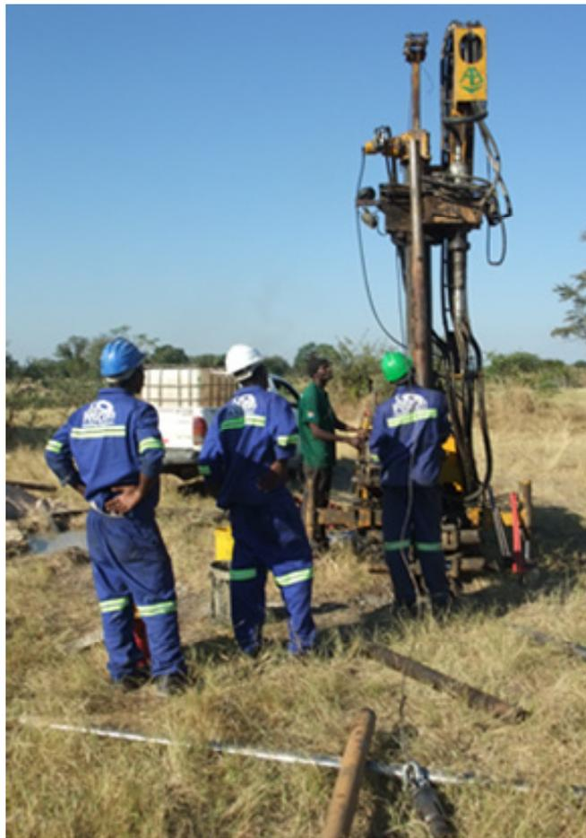
**Fig. 8:** Borehole core drilling at the Kasaya site (RV 12-27, see Fig. 2 for location) for sediment characterisation and geochronology.
