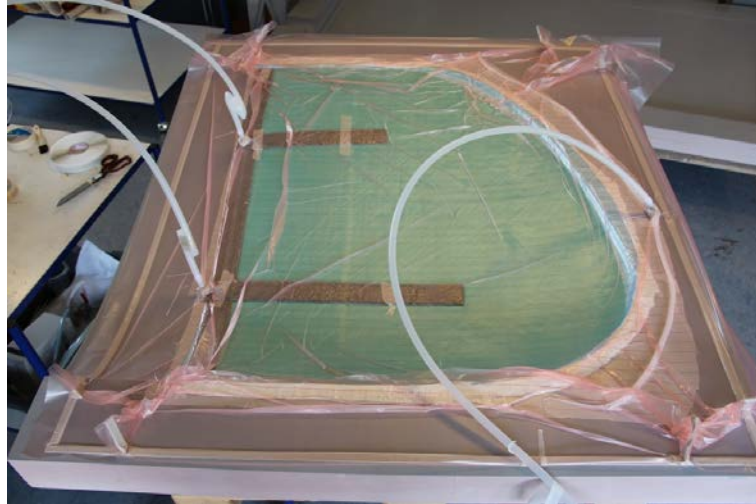
Figure 20 - Vacuum bagging of side pod.
