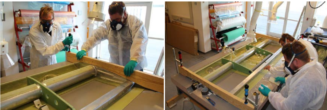
Figure 32 – Left: Fixation of aluminium structure. Bondline thickness was obtained using spacers. Right: Aluminium structure was aligned in the mold by the special design of the tube support in each end. Excess adhesive was removed when the structure was in place.
