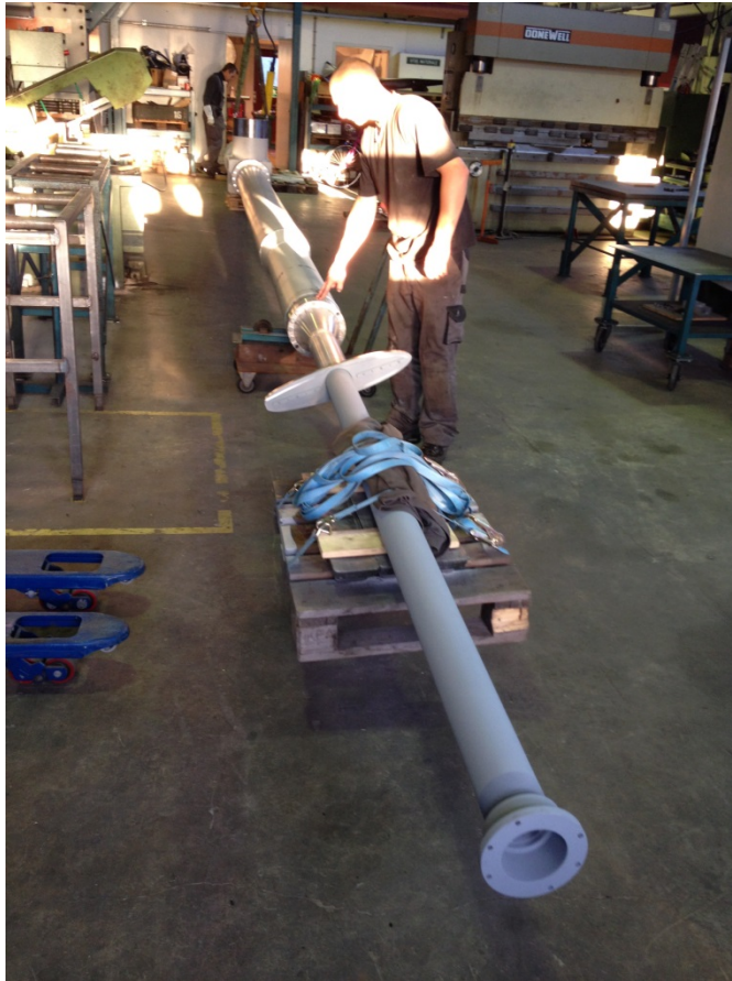
Figure 10 - Balancing of the boom.
