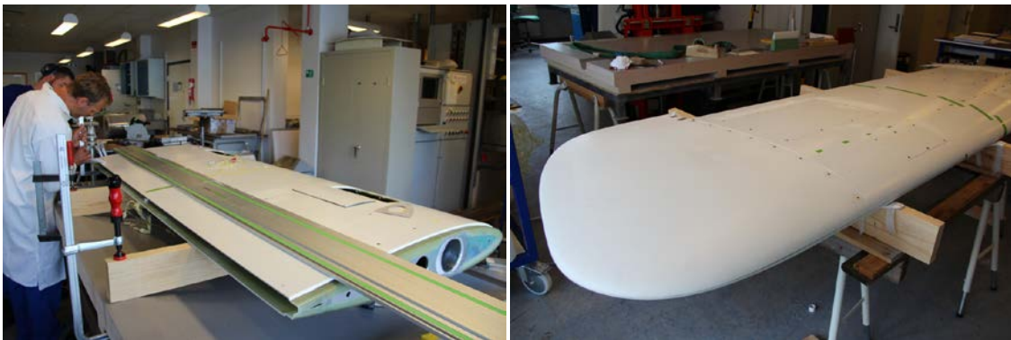
Figure 40 - Left: Laser lineup of laminate before cutting of trailing edge. Right: Mounting of side pods to wing section using helicoils in the aluminum spante. Good fit between wing section, side pods and hatches.
