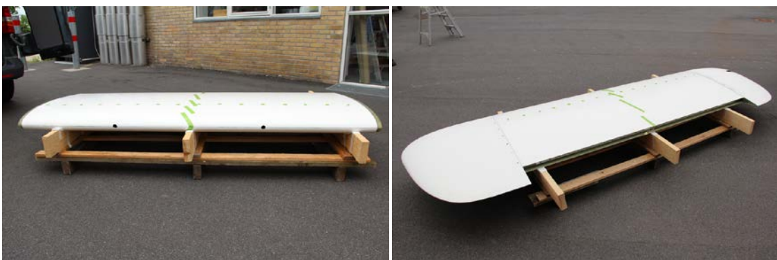
Figure 41 – Left: Holes for mounting of pitot tubes in leading edge. Right: Blade section with mounted side pods had a total weight of 96 kg before devices and rubber trailing edge was mounted.
