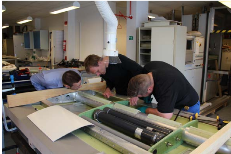
Figure 28 - Mounted V-profiles on top of the aluminum tube. Position of bondlines were marked together with positions of the U-profile overlap at the leading edge.
