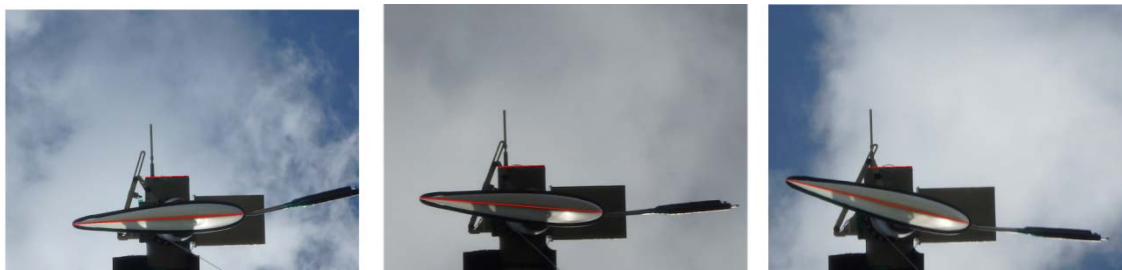
Figure 58 – Images for pitch calibration (pitch command signal 0-6V).
