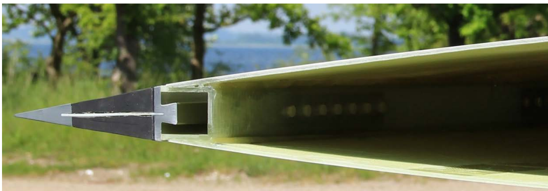
Figure 43 – Blade section mounted on boom.
