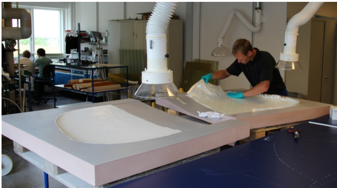
Figure 19 - Side pod mold with applied gelcoat (left) and lay-up of glass fabric on top of gelcoat (right).
