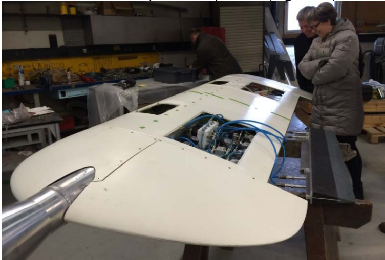
Figure 42 – Blade section mounted on boom.
