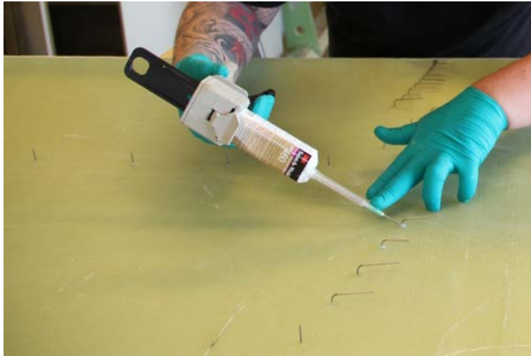
Figure 26 - Pressure holes were drilled in the shell at specific locations. Stainless steel rods were mounted with first cyanoacrylate and subsequently by an epoxy adhesive.
