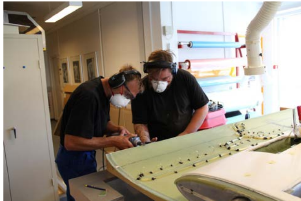
Figure 34 - Trimming of leading edge before assembly using a high speed drill .
