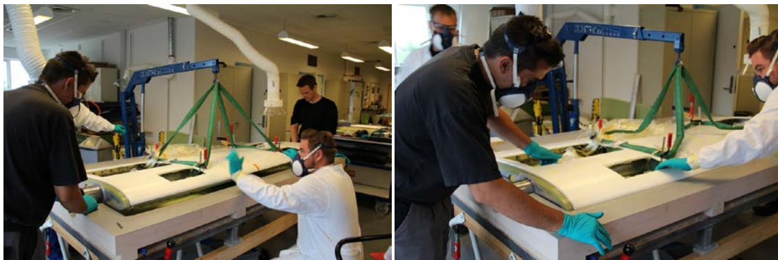
Figure 38 - Tube steering was used for fixation of components during assembly.
