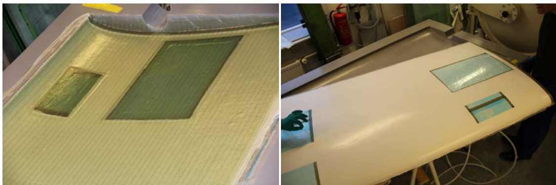
Figure 25 – Right: Close up of hatches casted into the laminate in order to obtain perfect fit. The holes for the hatches were cut afterwards. Right: Hatches covered with release foil were carefully removed and labelled.
