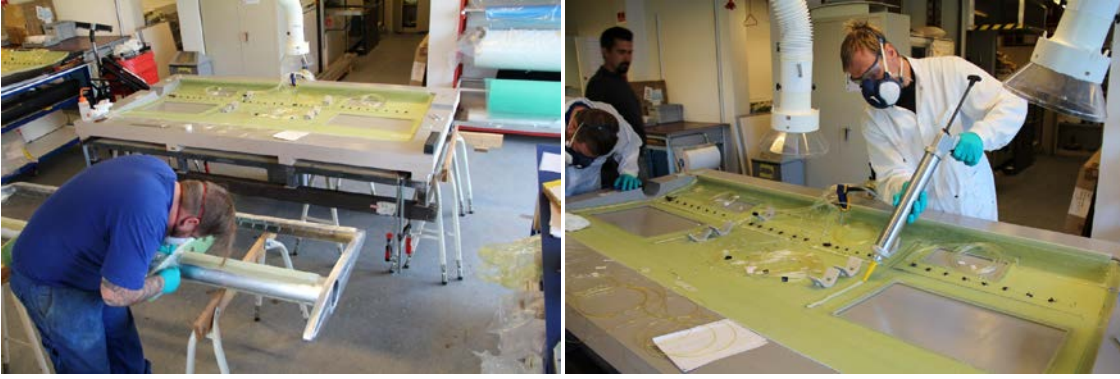
Figure 30 – Left: Preparation of aluminium part. Right: Placement of adhesive in the marked bond lines using a glue gun.
