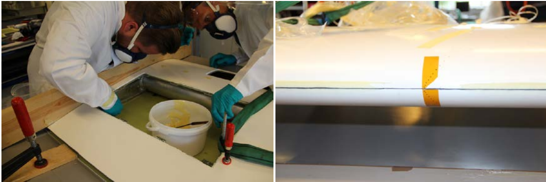
Figure 39 – Left: Removal of excess adhesive. Right: Pressure holes were covered with tape during the bonding to prevent them from being blocked.
