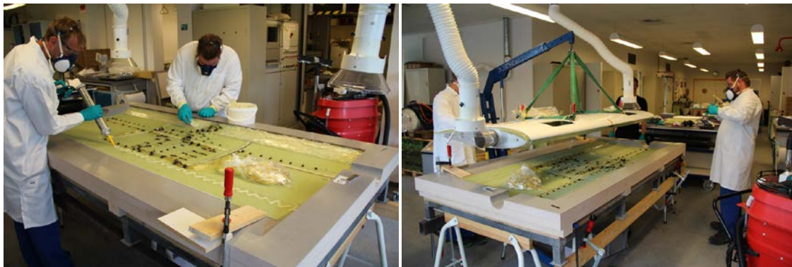
Figure 37 – Left: Adhesive being spread out in the marked bondline areas of the shell placed in the mold. Right: Top part mounted in a portable crane for easy and controlled joining of the parts.
