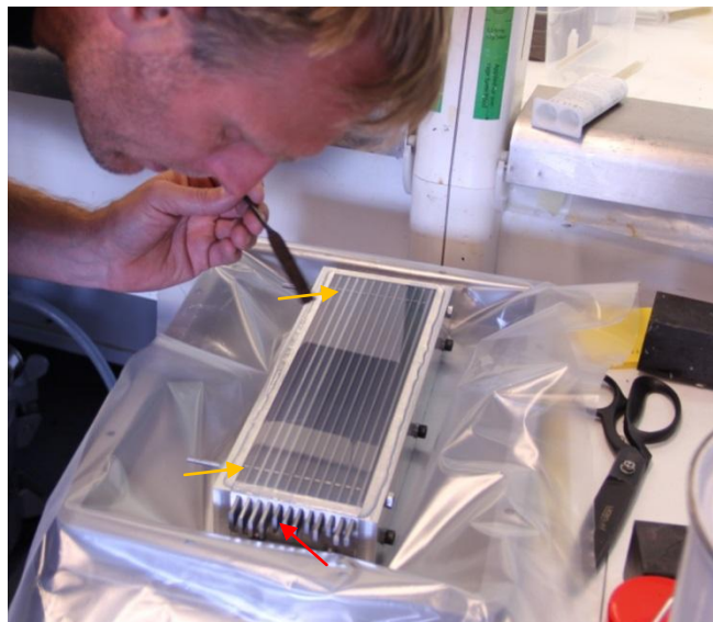
Figure 19 Mold for casting of active rubber flap parts with spanwise voids. Inlet holes for voids were casted in both ends, see yellow arrows. Manual removal of air bubbles in the resin before a top plate close the mold. The rods forming the voids are sticking out of the end flange of the mold, red arrow, making it possible to grab and remove them from the cured specimen.
