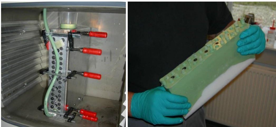
Figure 6: Vacuum casting of CRTEF part. To the left, the green rubber material is visual in the tube connection and in the outlet reservoir at the top of the mold inside the vacuum chamber. To the right is shown the cured specimen before trimming of excess material.
