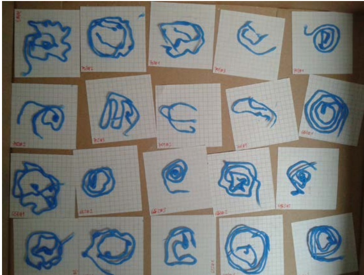
Figure 4 Collection of extruded samples with paraffin wax
