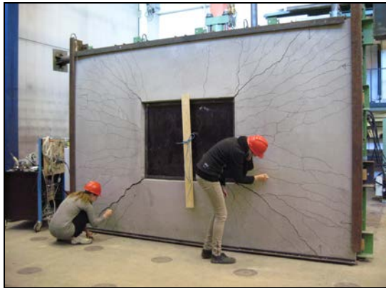
Figure 1 – Marking cracks in a tested wall element J and the load-displacement curve. Red starts indicate rupture of reinforcement /Sadiki and Reenberg, 2013/, /Youtube, 2013/.
