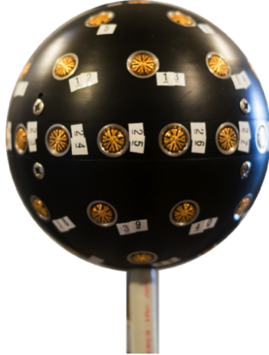
Figure 5.2: The 52-channel, mixed-order ambisonics microphone array investigated in this study.
