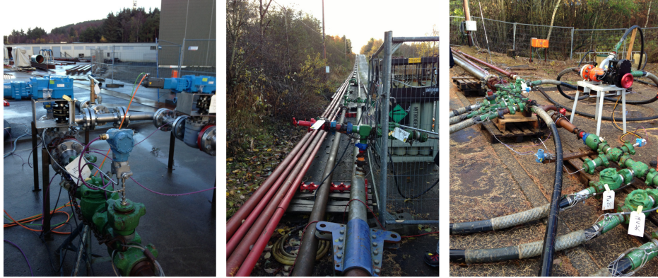
Figure 2: Experimental flow loop with choke manifold to the left, gas influx and washout emulation in the middle, and bit and loss emulation to the right.
