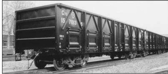
Fig. 7. A 4-axle Chinese hopper wagon.
