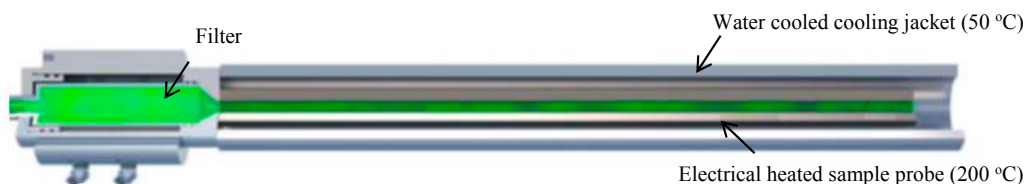
Figure G-2: Schematic drawing of the applied extraction probe (FSLmidth A/S 2012a).
