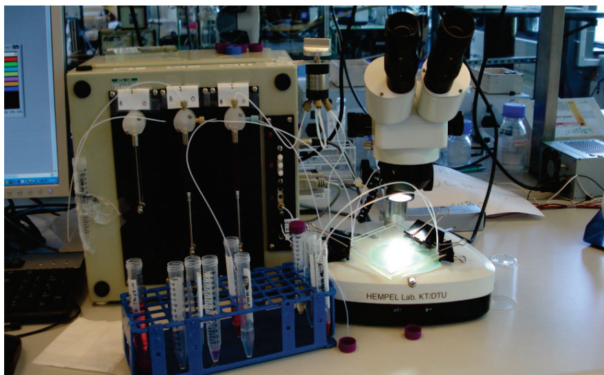
Fig 1b-1: Set-up showing the modular digital pump, the microscope and a microreactor
