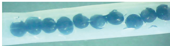
Fig 5.7: Tube (1mm ID and 8.5mm in length) with resin particles
