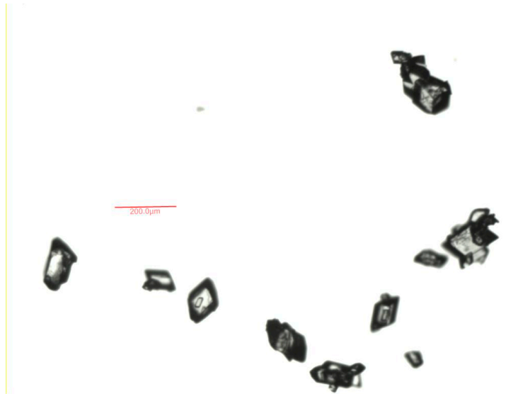
Figure 6.14: Pictures of the crystals in the sample withdrawn from the operation. The crystals have been dried and some agglomeration may have occurred in the drying process. Signs of inclusion appear present. A similar sample was drawn 10 min. later. This sample is shown in Figure 6.15
