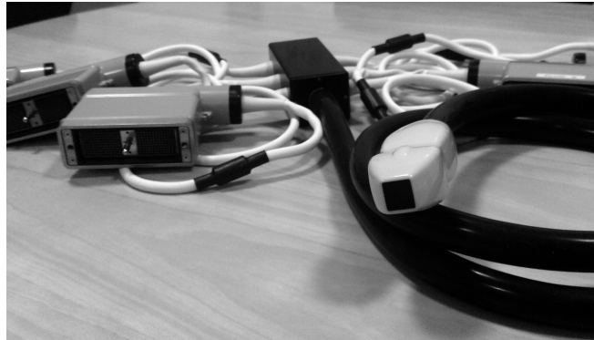
Figure C.11: The 32×32 element phased array ultrasound probe used for the measurements and modeled in the simulations.
