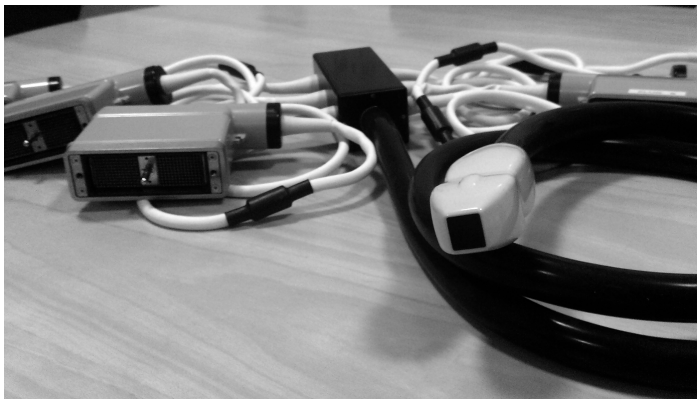
Figure 2.11: The 32×32 element phased array ultrasound probe used for the measurements and modeled in the simulations. The image is from paper C.
