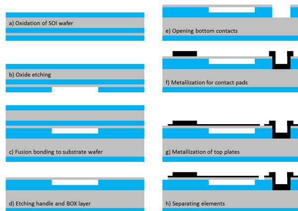
Fig. 1. Process steps for fabricating 1D arrays using fusion bonding and oxidation of both SOI and substrate wafer. Both top and bottom electrode can be contacted from the front side of the device.
