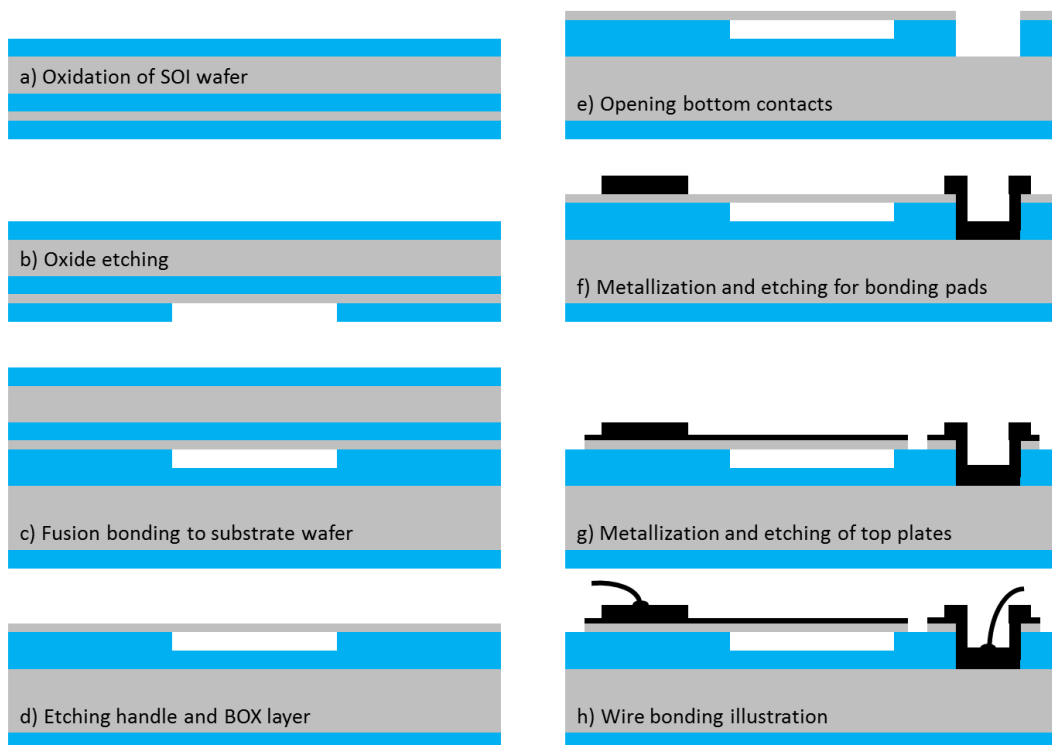
Figure 4.6: Process flow overview for the fusion bonding process made at DTU. a) Oxidation of both SOI and substrate wafer; b) defining cavities on SOI wafer by dry etching of the oxide; c) fusion bonding of the two wafers; d) removal of handle and BOX layer of SOI by etching; e) opening up to the bottom electrode by etching; f) defining bonding pads by metal deposition and wet etching; and g) defining top plates and contacts by metal deposition and wet and dry etching. j) The finished device after dicing and wirebonding.
