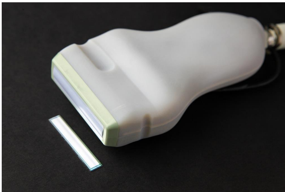
Figure 6.5: First finished TABLA probe with a similar device in front of it.
