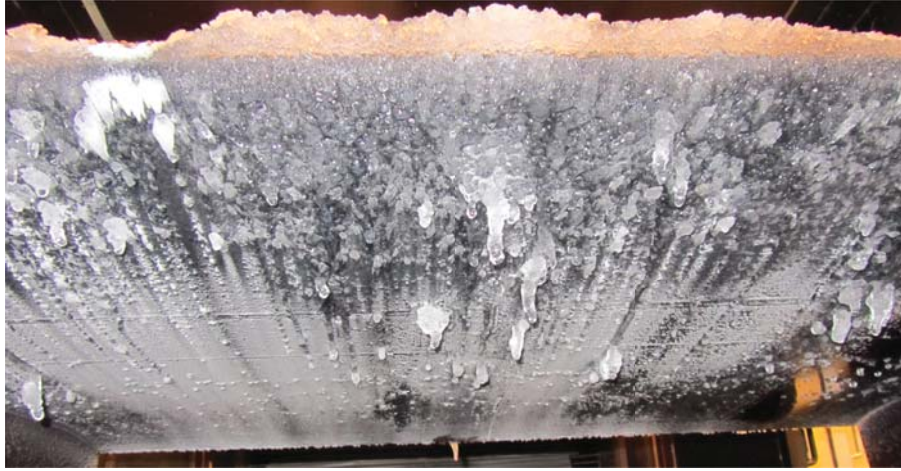
Figure B.2: Glaze iced pressure side of the airfoil for \alpha = 7^\circ .
