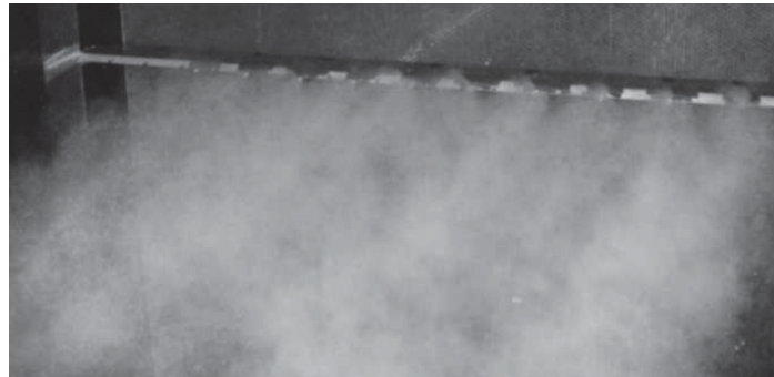
Figure 2. Spray system produces cloud in the wind tunnel.
