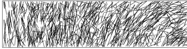
Figure 1.3: Top view of a beam specimen cut from a slab made of fibre reinforced self-compacting concrete (see Section 7 for further details). Individual lines were obtained by x-ray computed tomography and represent immersed steel fibres.
