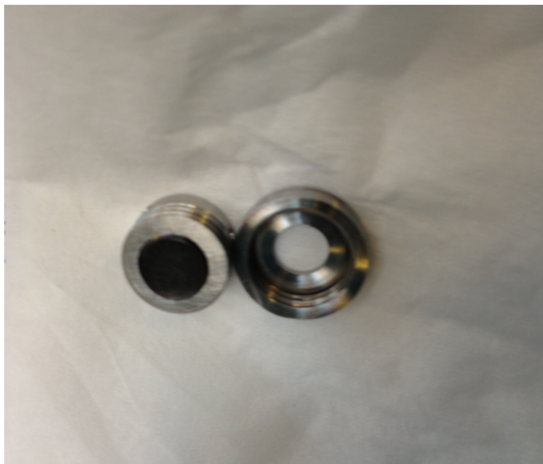
Figure 2.3: The picture shows the sample holder for investigations of powder catalysts.
