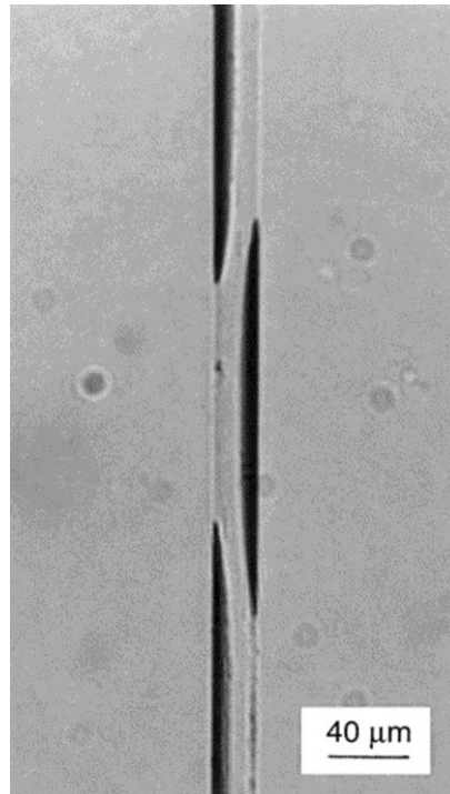
Figure 2.12. Partially debonded fibre caused by the transverse load (applied in the direction perpendicular to the fibre) [7]. The viewing direction parallel to the fibre direction is not suited for the precise debond angle measurements.
