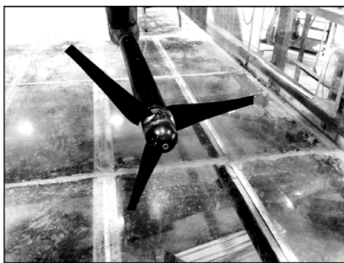
Figure 1. A windmill rotor model in an empty water flume
