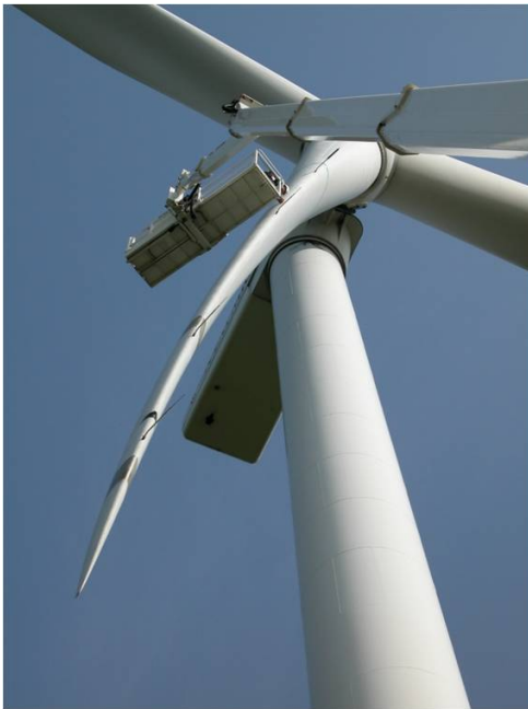
Figure 1. The blade of the NM80 turbine equipped with measurement devices.
