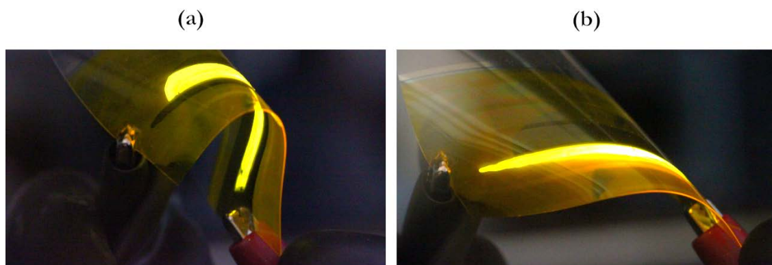
Figure 7.1: (a, b) Photographs of the light emission from two slot-die coated LEC devices driven at V = 7 \text{ V} illustrating the bi-directional light emission and the device conformability. Reproduced with permission from Nature Publishing Group [2]
