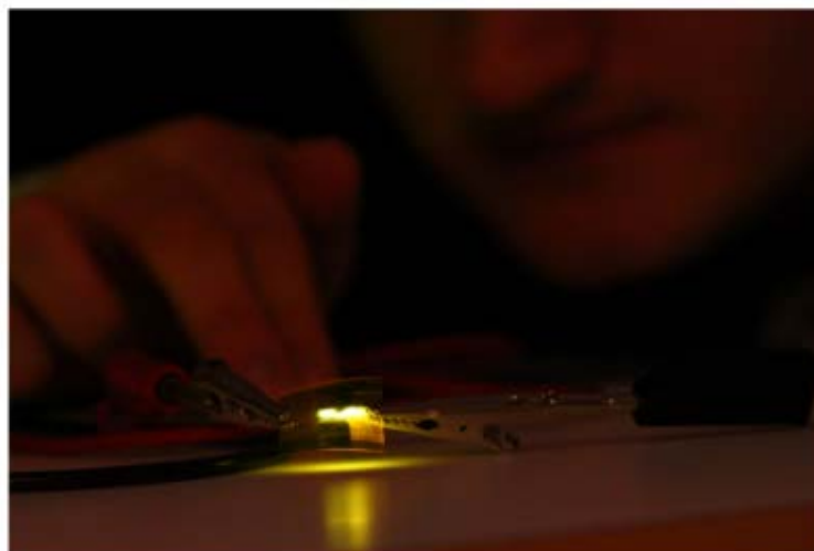
Figure 7.7: Photograph of an encapsulated roll-coated device operating at V = 7\text{ V} under ambient conditions. Note that the device had been stored under ambient air for 3 days before the voltage was applied.
