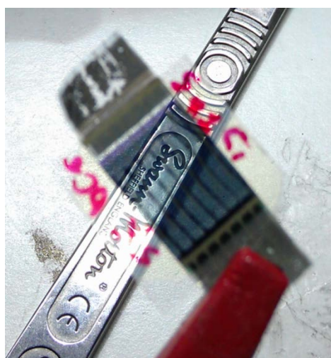
Figure 5.14: Semi-transparent tandem solar cell consisting of the 12 layer stack with active layers of PDTSTTz-4:PCBM and PSBTBT:PCBM.
