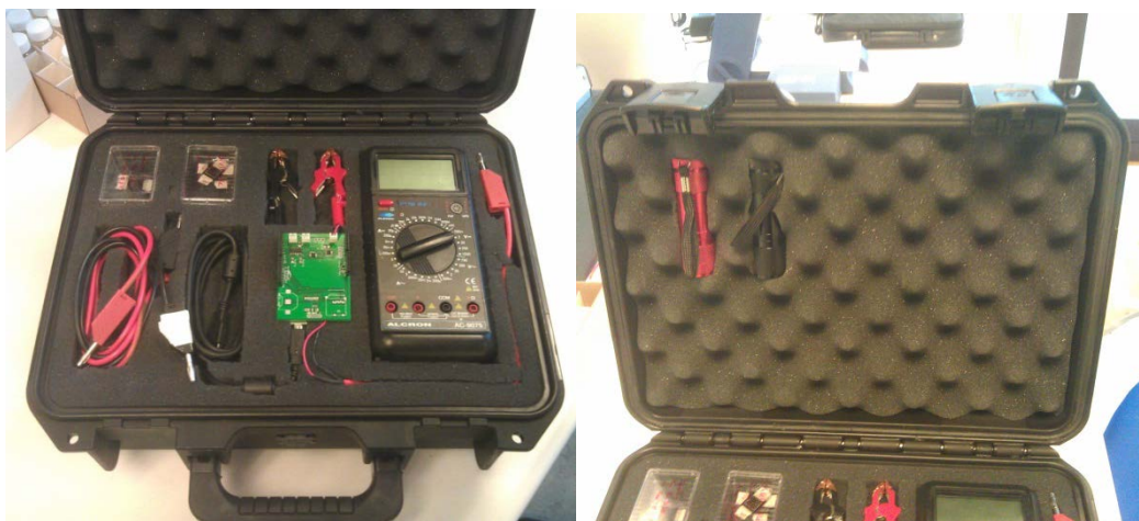
Figure 8.6: Double sided illumination tandem solar cell demonstration. A rugged case with two LED torches, a multimeter, wires, crocodile clips and an Arduino with the measurement board attached. The case was developed to help demonstrate what and how the roll coated solar cells look and perform.
