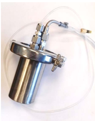
Figure 2.17: Pressure driven pump for supplying viscous PEDOT:PSS top layer ink. Pump is driven from the laboratory compressed air system with a 1.5 bar to 2 bar pressure.
