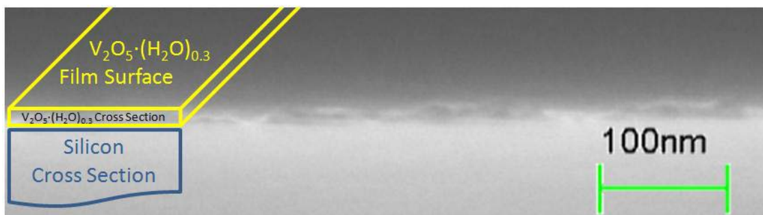
Figure 3.12: SEM cross section (tilted 17°) of 15 nm-thick cleaved V_2O_5 \cdot (H_2O)_{0.3} film on a crystal silicon substrate showing film thickness and uniform morphology on the film surface.
