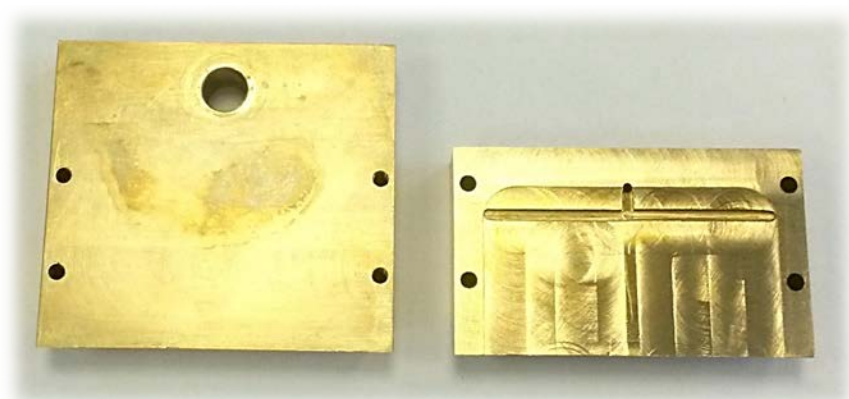
Figure 2.9: 50 mm head design. At the inlet a pressure distribution channel has been milled into the head to even out the pressure across the width of the bottom outlet. This head also has a support beam in the center similar to the 25 mm head.
