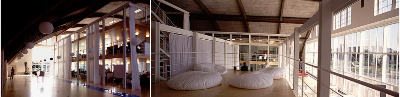
Figure 10 Left: The three floors with offices are placed at a distance from the facades, and are surrounded by large curtains that create room in rooms. Right: On the top floor, spaces for rest have been created. Photographs: Per Munkgaard Thorsen, www.arkitekturbilleder.dk
