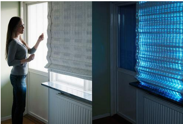
Figure 26 The Energy Curtain. Left: During the day, the curtain harvests energy from the solar cells placed on the side of the curtain facing the outside. Right: At night, the curtain becomes a light source thanks to optical fibres woven into the curtain and LEDs (light emitting diodes) that emit light that is then transported and emitted through the optical fibres. The curtain only lights up when the amount of daylight outside is too low. Photograph: Carl Dahlstedt. © Interactive Institute.
