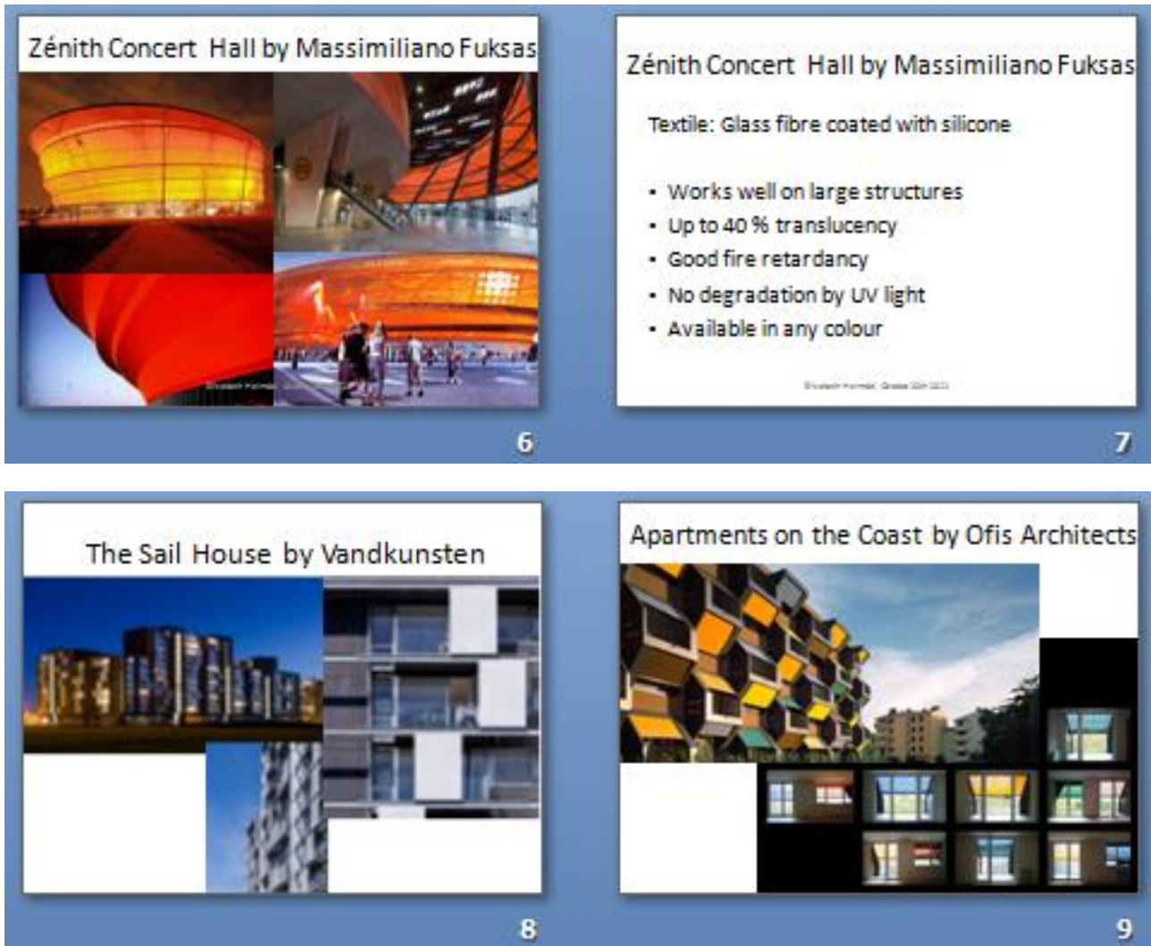
Figure 77 Examples presented in Power Point presentation. The presentation of each specific textile started with the presentation of a specific building (slide 1 and 6). Details were then provided about the specific textiles (slide 2 and 7), before a couple of other examples of architectural uses of this material were shown (slides 3, 4, 8 and 9). Photographs found on the internet, on respective architects' website or material suppliers' websites.
