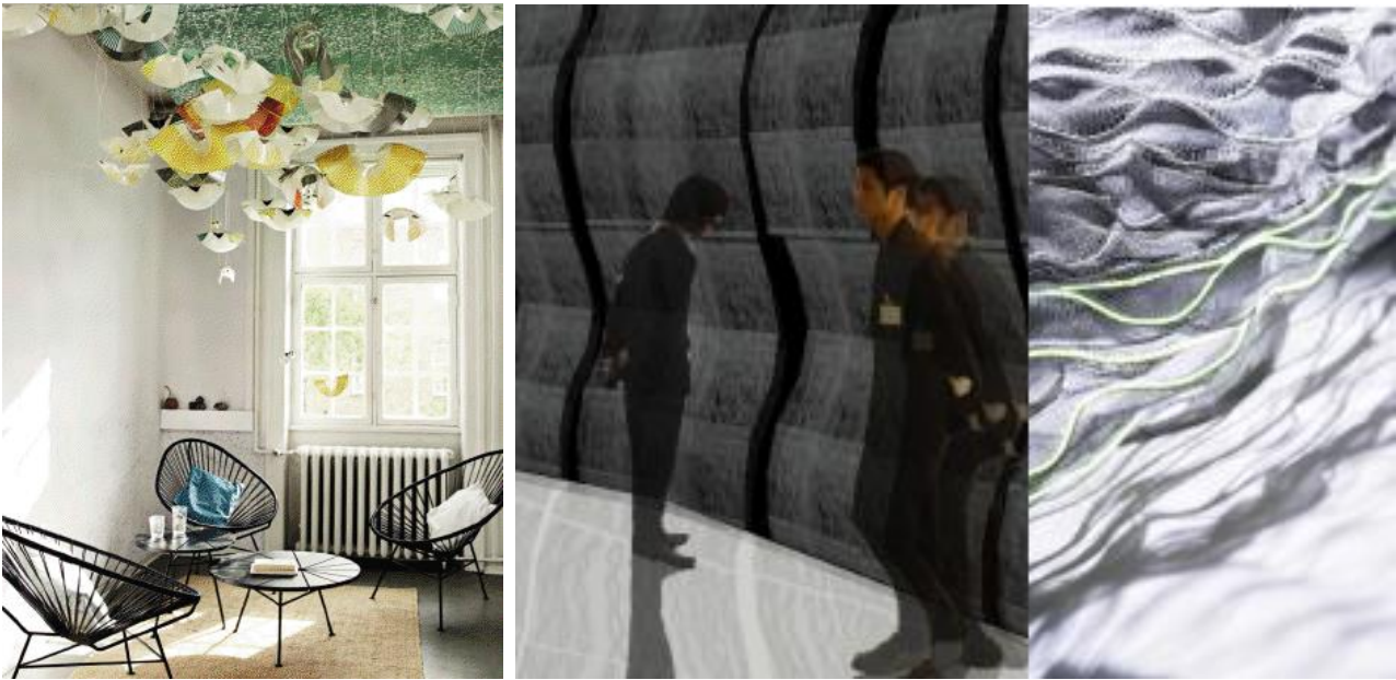
Figure 29 Left: The ceiling structure Reef by Aurélie Mossé and collaborators. Each module consists of electro-active polymer that contracts when subjected to an electrical impulse. This contraction is amplified by the design of the “wings” attached to the polymer. Photograph: © Anders Ingvarsten, with kind permission from Aurélie Mossé. Centre and Right: Rendering and prototype of “knitted light”, an interactive textile wall that reacts to the persons in the room by displaying different light patterns. Source: (Dumitrescu, 2011b, p. 41).
