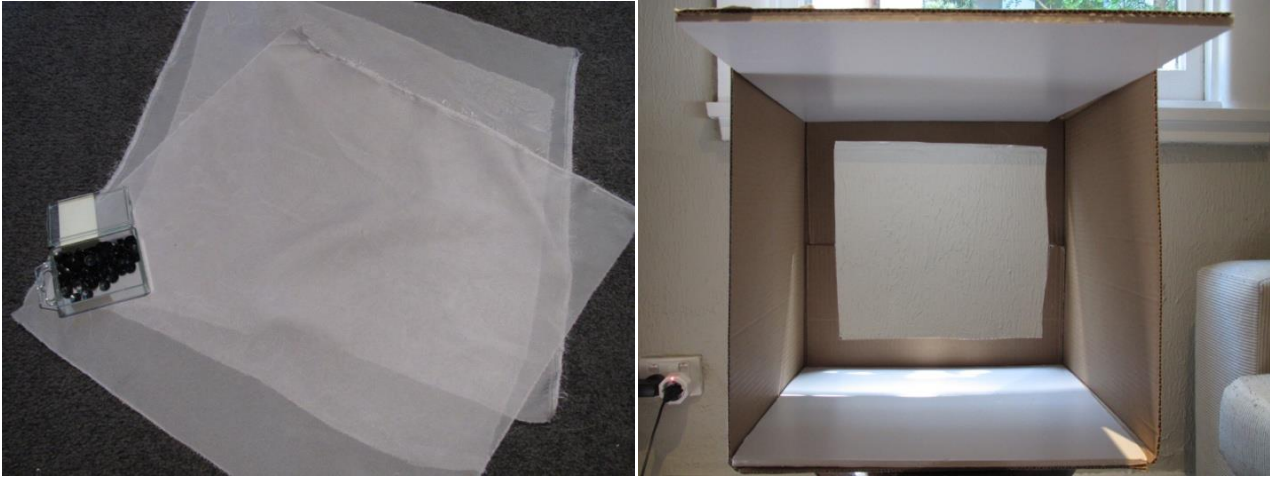
Figure 97 Left: Three square pieces of grey polyester chiffon. Right: Cardboard “room” with ceiling and floor covered in foam board. Photographs: © Elisabeth Heimdal.
