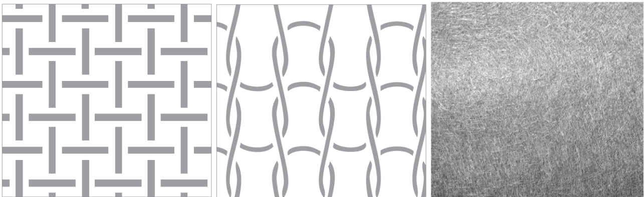
Figure 13 From left to right: woven fabric in plan weave, (weft) knitted fabric and non-woven fabric. Source: (Simonsen Degn et al., 2007, p. 8, 16 and 22).
