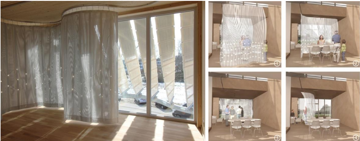
Figure 11 Left: View of room with partition curtains in which LEDs are integrated. The strips of solar cells are visible through the window. Right: Four ways in which the curtain, attached on an overhead rack, can be used to accommodate different needs. Photographs: © KVA.
