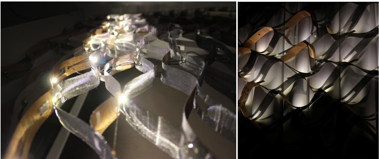
Figure 33 Left: View from above of prototype where LEDs are combined with textile strips. Right: View of the same prototype from the side. Photographs: © Astrid Mody.
