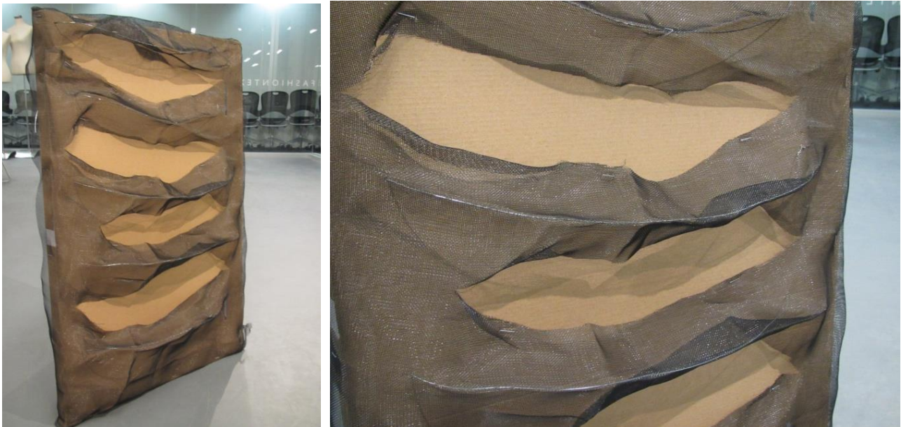
Figure 91 Model made by group 4. The windows are imagined placed in the openings in the textile, and the "visors" created by the curved wire covered with fabric provide shading. Photographs: © Elisabeth Heimdal.
