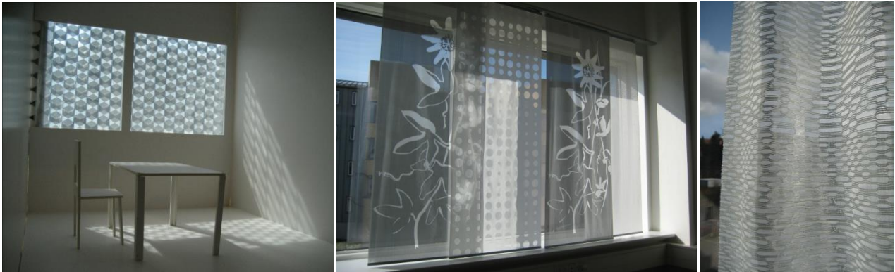
Figure 27 Left: Experiments at the scale 1:4 with aluminium fabric with dévoré pattern and aluminium foil. The aluminium foil is placed closest to the window and has heat reflecting properties. Centre: Experimental set-up with full-scale prototypes. The prototypes of screening solutions are panels with flower pattern or geometric patterns. Right: Hand woven fabric made with three fibres: Trevira CS filament, a polylactic acid yarn that is naturally UV-resistant and Waveron from Teijin (a special light reflecting fibre). Photographs: © Vibeke Riisberg, with kind permission.
