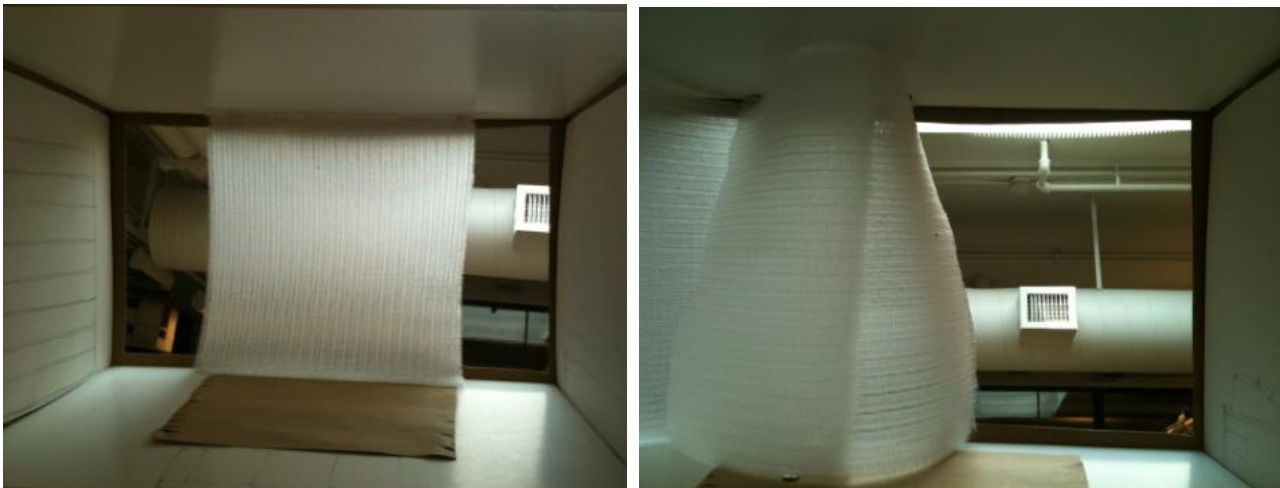
Figure 113 First trials by Felecia and David. Left: One piece of spacer fabric is attached horizontally in the opening of the box. Right: Two pieces of spacer fabrics are folded into each other. Photographs: © Felecia Davis.
