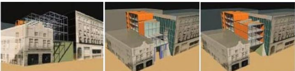
Figure 40 Images showing the variety of configurations allowed by the structure and the textile envelope in a temporary “trial” building. Left: Only the building furthest away from the street has an exterior envelope. Centre: One more building is now covered. Right: All the structures are now covered with an exterior textile envelope. Source: (Fernández, 2006, p. 72).
