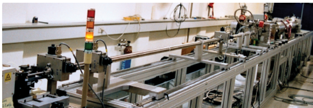
Figure 4.1: The SAXS setup at DTU Risø Campus operating in its long geometry. The rotating anode can be seen at the far left. The sample chamber, the flight tube and the detector can be seen to the far right.
