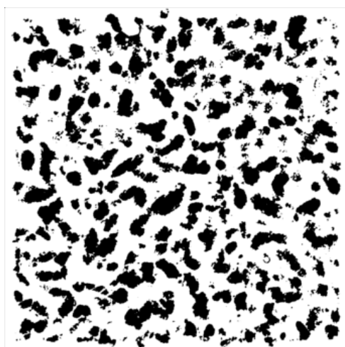
Figure 5.8: By further using a median filter, with a 5 \times 5 kernel on figure 5.7 a lot of the shot noise is also removed
