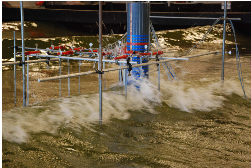
Figure 72: Breaking wave impact at scale 1:36.6.
