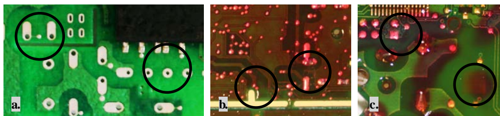
Figure 6: Selected areas for optical microscope pictures, of a) reflow b) wave and c) selective wave soldered and coated PCBs
