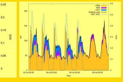
The Studio 14 feeder was modeled in detail using OpenDSS, a distribution system simulator developed by the Electric Power Research Institute. The four schedulable facilities were connected electrically to the Studio 14 feeder, in addition to a background load obtained from data provided by the utility. The outputs of the simulation include voltage, current, power, phase at any location on the feeder. Voltage at one of the nodes was used here as an indicator of power quality.
