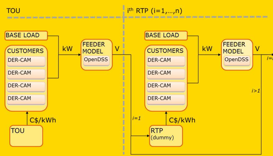
The iterative scheme used here progressively incorporates the collective effects of individual "greedy" individual optimizations. The simple form of the RTP also retains memory from previous iterations to maintain stability.
