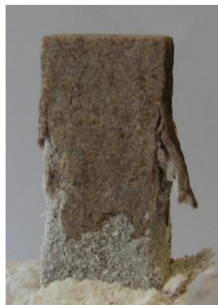
Figure 5: Subflorescence. Nexø sandstone exposed to Na 2 SO 4 solution
