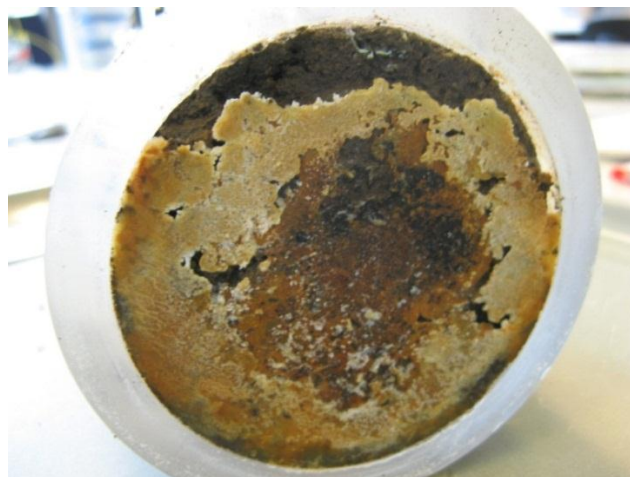
Figure 2: Cathode end of the soil sample after EDR on Soil 2, when the cation-exchange membrane was removed.
