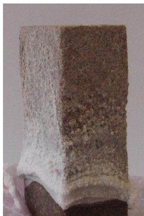
Figure 4: Efflorescence. Nexø sandstone exposed to NaCl solution.
