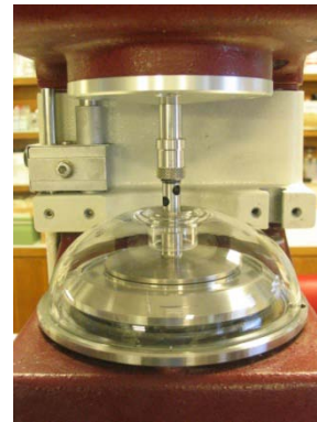
Figure 2.9: The rotational rheometer HAAKE RheoStress RS-150™ equipped with a solvent trap.
