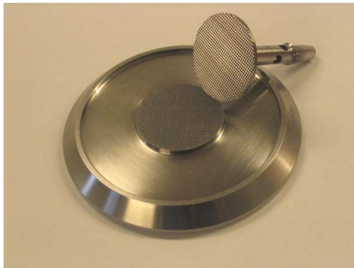
Figure 2.8: Parallel plates system. The rotor and the plate surface have a milled surface to improve the contact with soft materials.
