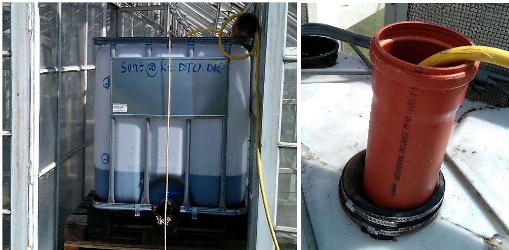
Figure 6: Mobile low-tech AD demonstration unit and feeding tube, designed as part of the study (Thomsen and Heiske, 2012, unpublished and not part of any current manuscripts).
