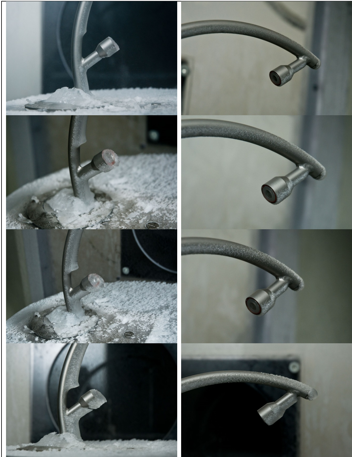
Figure 7 Ice build-up on non-heated sonic sensor heads on lower (left) and upper (right) sonic sensor heads. From top and down after 20min, 40min, 50min and 60min, respectively.
