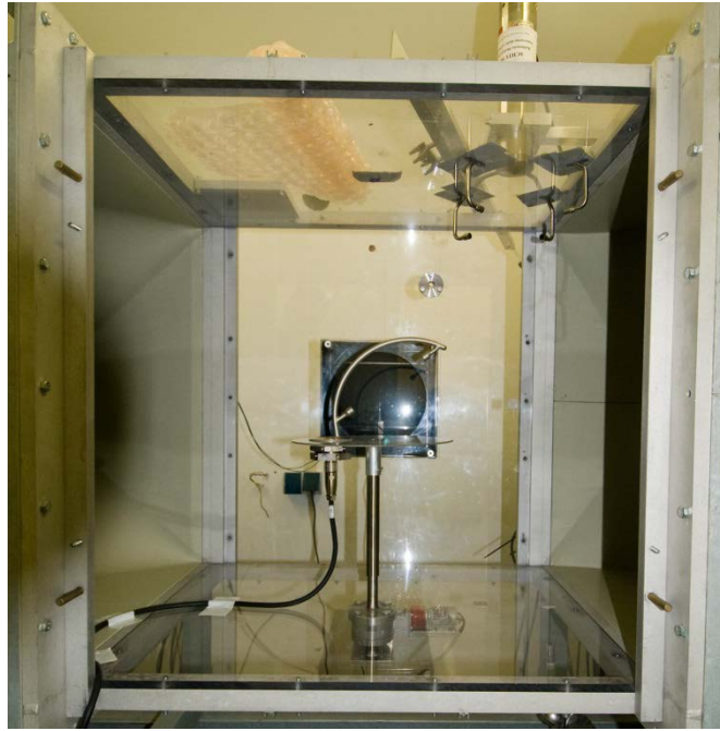
Figure 3 Setup of spinner anemometer sonic sensor in climate wind tunnel with flow from the right. At top is mounted a heated 2D Thies sonic for reference wind speed
