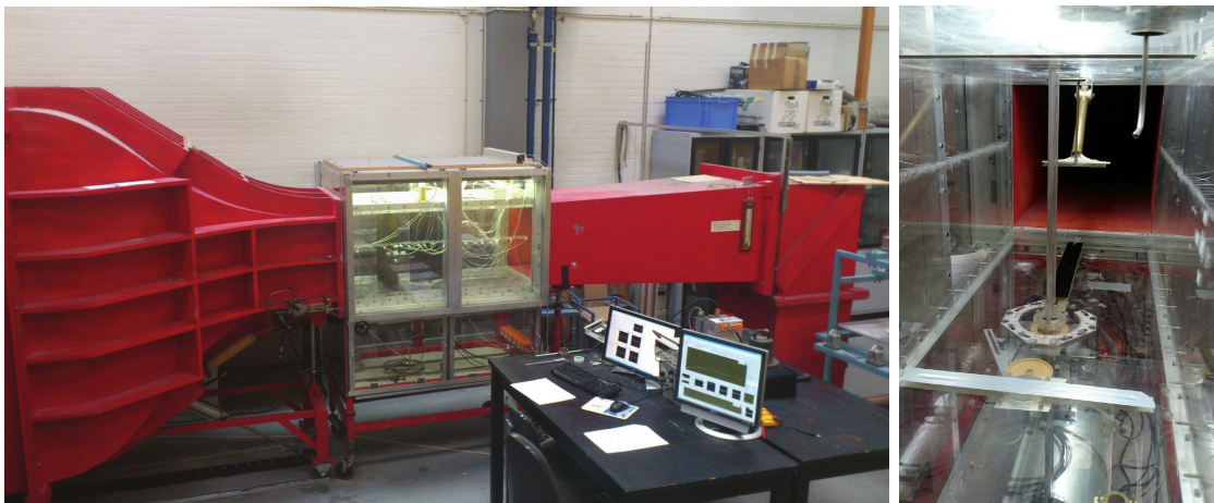
Figure 4.2: Wind tunnel facility at the Technical University of Denmark (left) and the test section of the wind-tunnel (right) showing the vertically mounted airfoil, pitot tube, and wake-rake.
