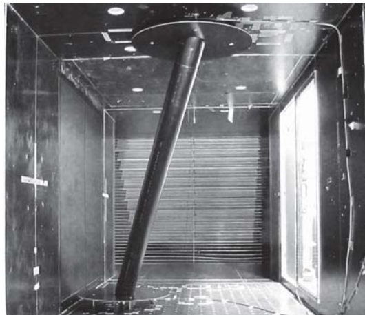
Figure 4.6: Inclined test configuration in static conditions.
