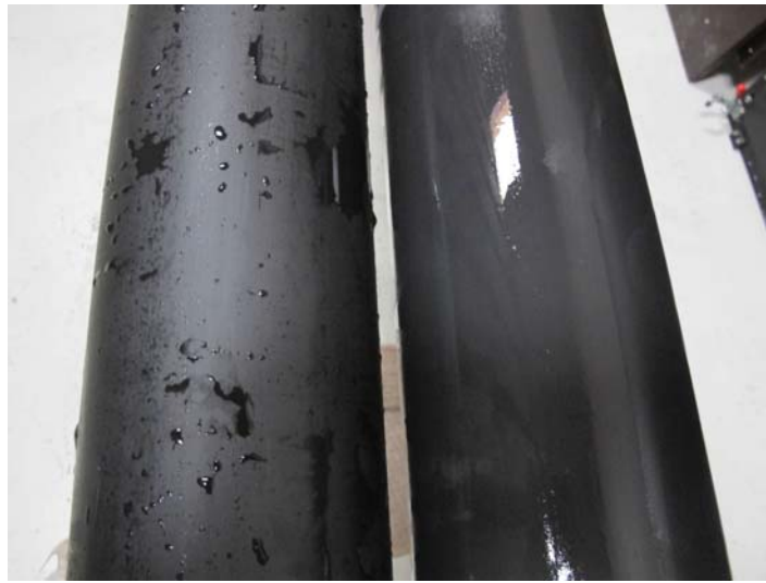
Figure 5.1: Effect of polyvinyl coating: untreated cable to the left compared to newly treated cable to the right exposed to water spray.
