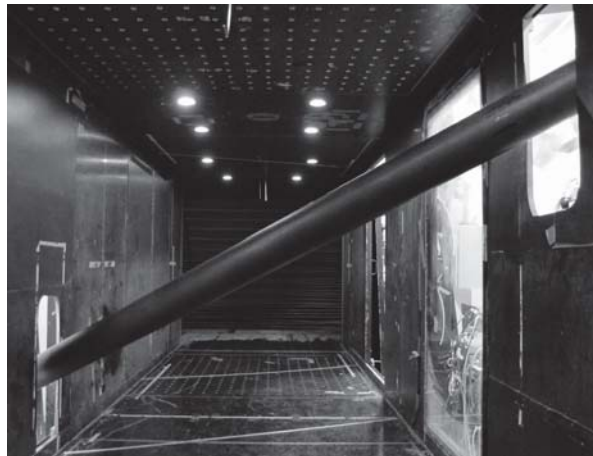
Figure 4.2: Cable model seen from the inside of the wind tunnel test chamber.
