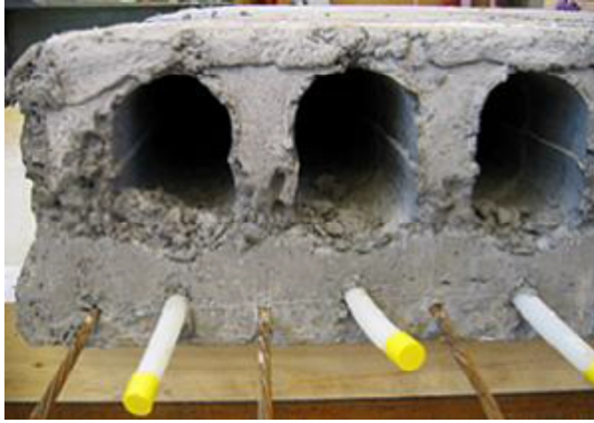
FIG 2. Concrete hollow deck with integrated PEX pipes
