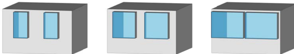
Figure 1: Illustration of glazing-to-floor-ratio for a 4m x 4m room. From left to right: Glazing-to-floor ratio of 15%, 25% and 35%.
