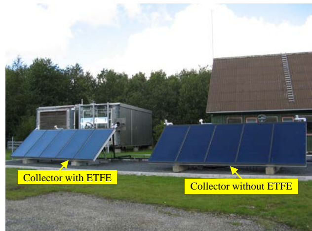
Fig.1 Photo of two HT solar collectors for tests
