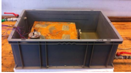
Fig. 2. Plastic tub for thermostatic bath with pipe connections and steel box.
