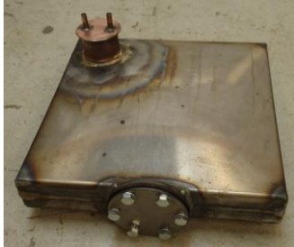
Fig. 1. 302 x 302 x 55 mm steel module containing a salt water mixture.
