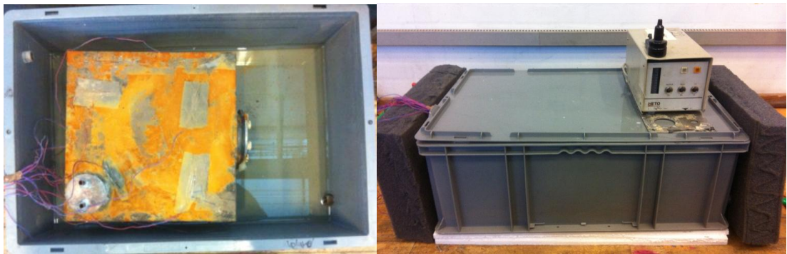
Fig. 3 (a). Top view of thermostatic bath with steel box. (b) Thermostatic bath with lid and thermostatic controller.
