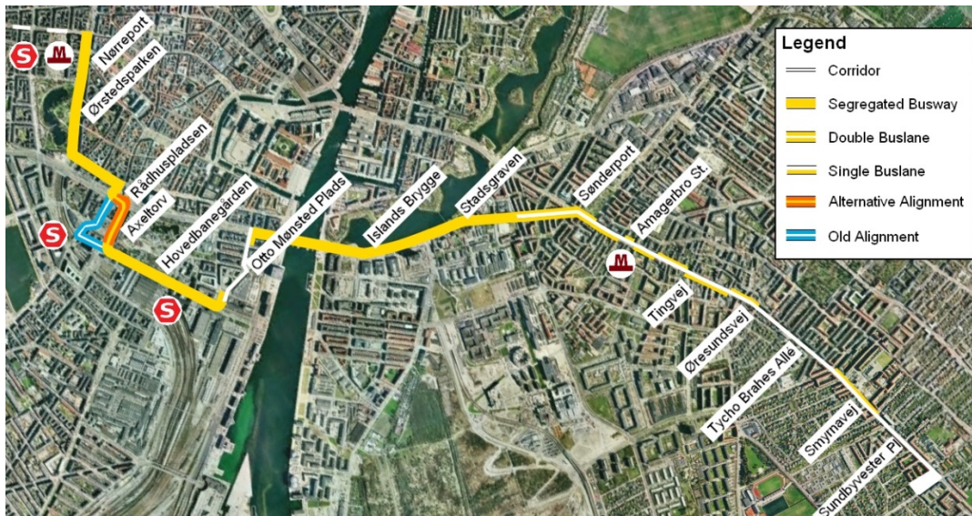
Figure 7: The layout of the proposed BRT upgrade of the 5A corridor between Nørreport station and Sundbyvester Plads.
