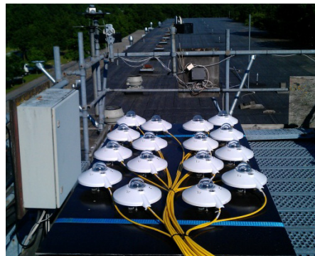
Fig. 3. The 16 pyranometers mounted on horizontal for side-by-side “calibration” measurements.
